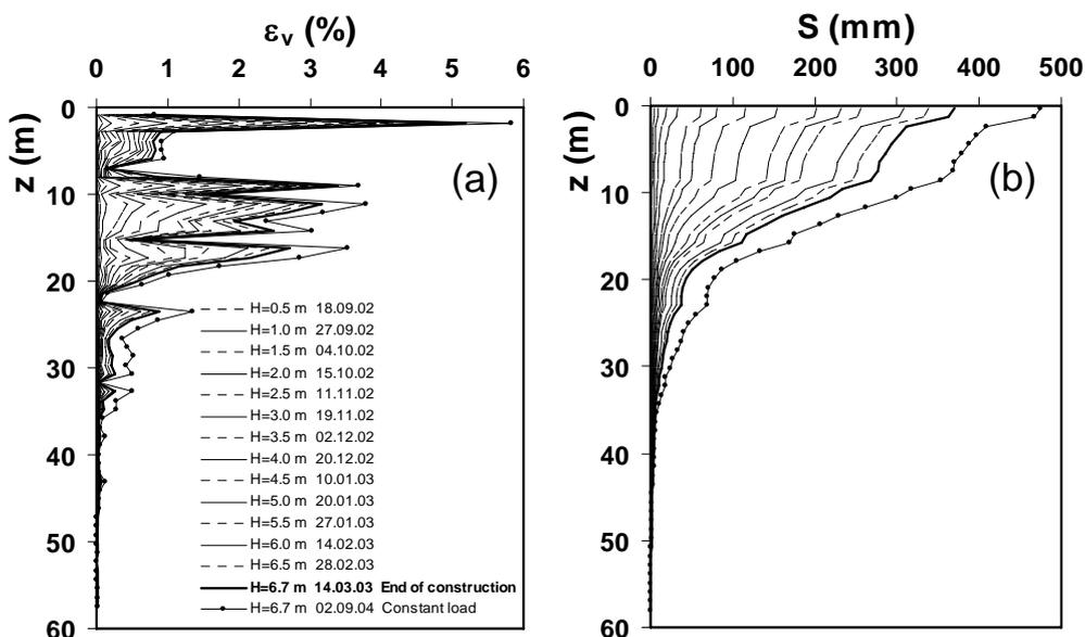
Fig. 13. (a) Vertical strains measured every 1 m depth under the center of the embankment and (b) corresponding accumulated settlements (updated after Simonini 2004)
