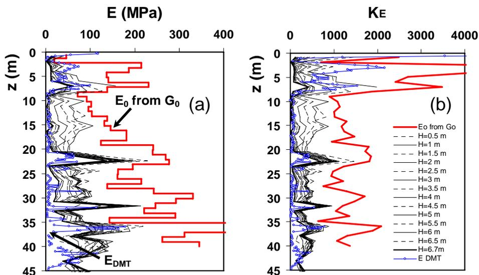
Fig. 17. Variation of (a) secant Young's modulus  $E$  backcalculated from vertical strains measured under the center of the embankment under various loads throughout embankment construction and (b) corresponding modulus number  $K_E$
