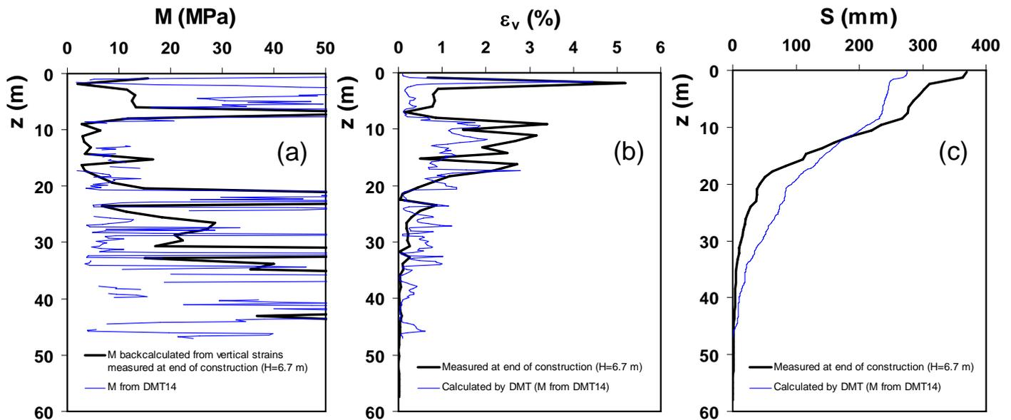
Fig. 16. Comparison of (a)  $M_{DMT}$  vs  $M$  backcalculated from measurements, (b) vertical strains  $\epsilon_v$  and (c) accumulated settlement  $S$  measured under the center of the embankment at the end of construction and calculated by  $M_{DMT}$
