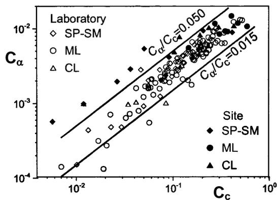
Fig. 12. Ratio between secondary and primary compression indexes  $C_\alpha/C_c$  obtained from laboratory and from observed full-scale strain-time curves (Cola & Simonini 2005)
