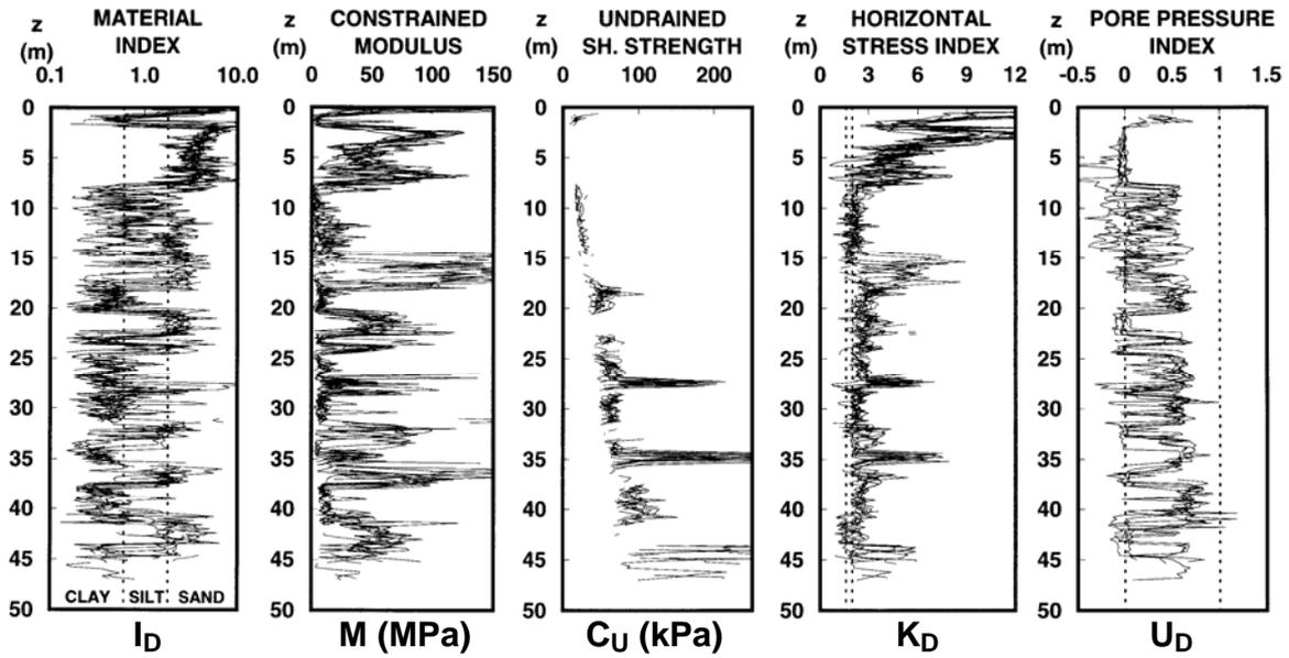
Fig. 3. Superimposed profiles of all DMT soundings (DMT 11, 12, ..., 20)
