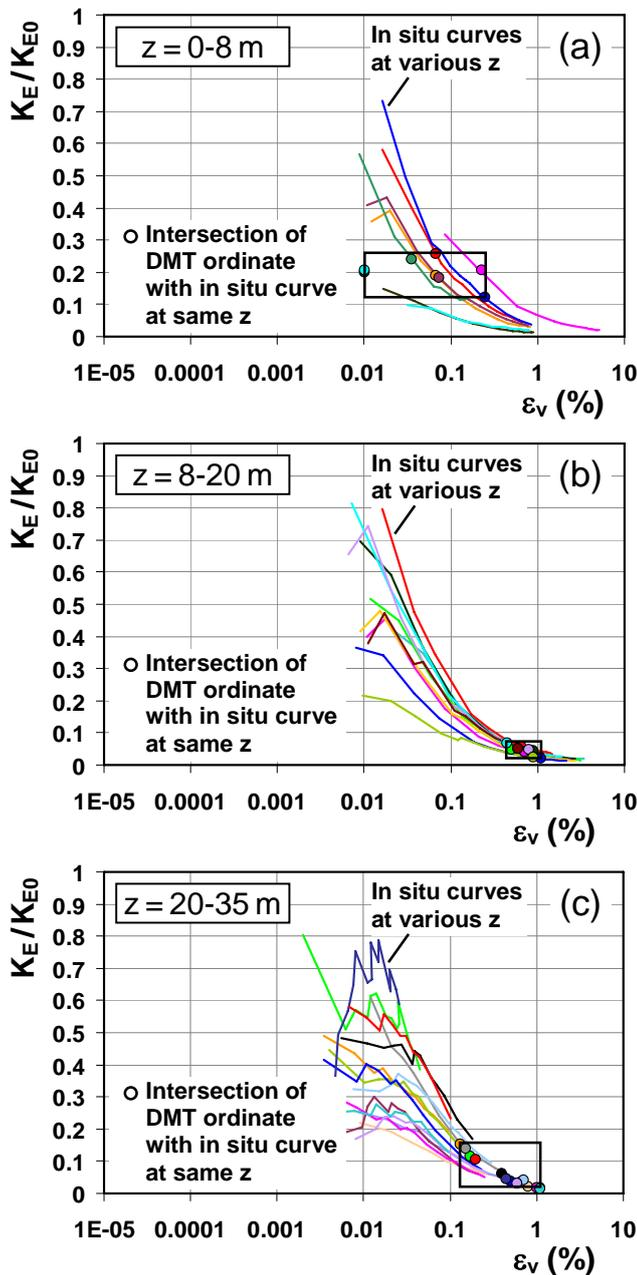
Fig. 18. Curves of decay of soil stiffness with vertical strain backcalculated from measurements (curves labeled "In situ curves") and their intersection with datapoints corresponding to DMT moduli  $M_{DMT}$  at the same depth
